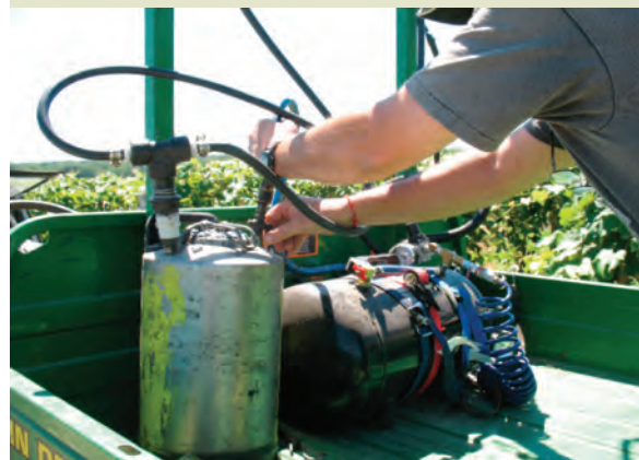
Fig. 4. Gator-mounted mechanical applicator for treatment of vineyards with SPLAT-GBM. Width of the applicator boom can be adjusted for different trellis systems and row spacing (top). Close-up of refillable air tank and SPLAT canister (bottom).
